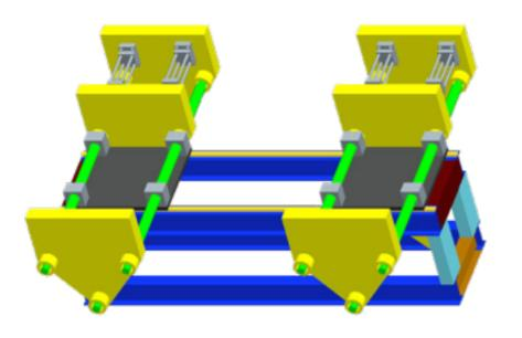
1. <u>Tiebarless (Patent) clamping</u> system:
